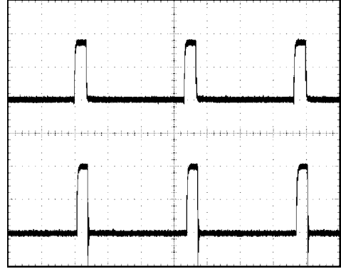
30kHz PWM Dimming (10% Duty Cycle ON)
